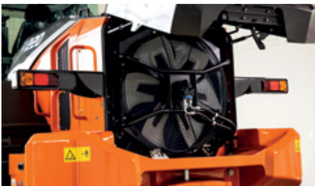
Intelligent fan operation system prevents radiators clogging.
