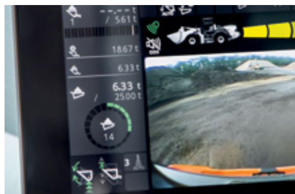
Work more productively and accurately using the payload checker.
